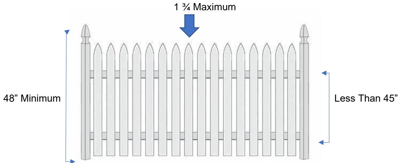
If horizontal planks are less than 45" part the vertical spacing can not be more than 1 ¾"
