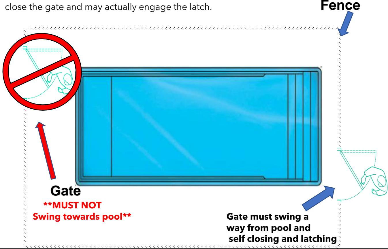
**48" high gates with latches mounted less than 54" from the ground**
