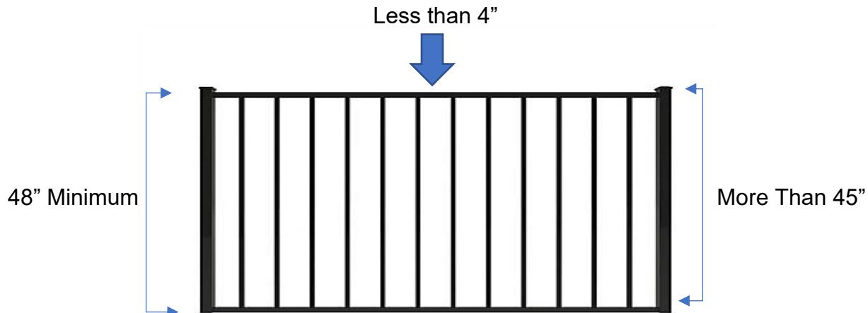
If horizontal rails are more than 45" part the vertical spaces cannot be more than 4" apart
